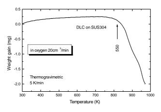
Fig.3 Thermo-gravimetric curve of DLC film in dry oxygen.
