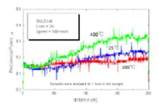
Fig.5 Effect of annealing temperature of DLC film on friction coefficient.
