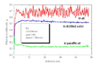
Fig.2 Friction coefficient of TiN film with various lubrications.
