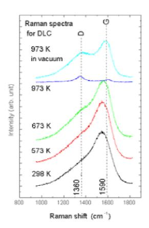
Fig.6 Raman spectra for DLC film after annealing at various temperature.
